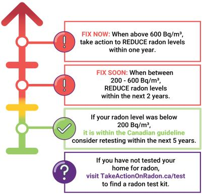
Since radon levels fluctuate over time. testing with a long-term test (of at least 91 days) provides a better estimate of your annual exposure. Many digital detectors are available to purchase or to borrow for shorter test durations, but we still recommend testing for at least 91 days. If you borrow a digital monitor for a shorter test, consider following up with a long-term test.
