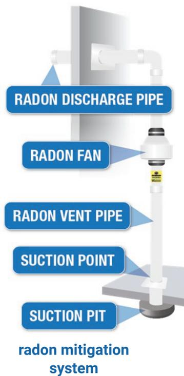
Radon gas levels are reduced the most by installing a **radon mitigation system**. Research shows that **certified radon professionals** can reduce levels by over 90%. Other steps, such as increasing ventilation and sealing cracks, can help in the short-term but are less effective.
