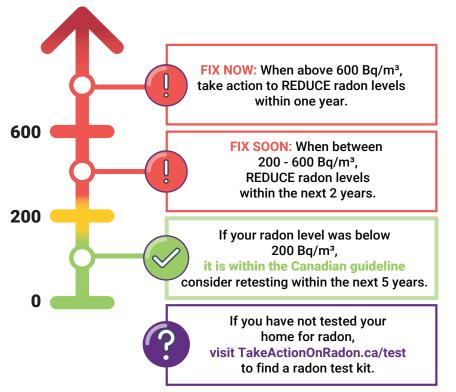
Since radon levels fluctuate over time, testing with a long-term test (of at least 91 days) provides a better estimate of your annual radon exposure. Many digital detectors are available to purchase or to borrow for shorter test durations, but we still recommend testing for at least 91 days. If you borrow a digital monitor for a shorter test, consider following up with a long-term test.
