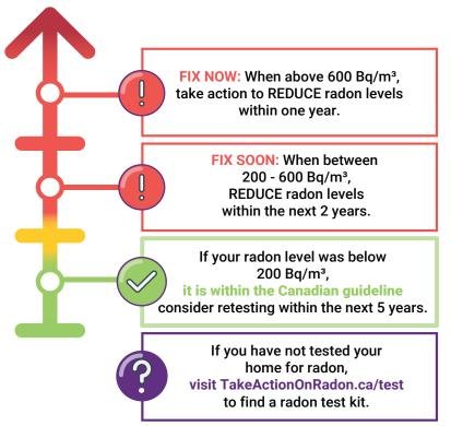
Since radon levels fluctuate over time. testing with a long-term test (of at least 91 days) provides a better estimate of your annual radon exposure. Many digital detectors are available to purchase or to borrow for shorter test durations, but we still recommend testing for at least 91 days. If you borrow a digital monitor for a shorter test, consider following up with a long-term test.
