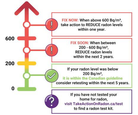
Since radon levels fluctuate over time, testing with a long-term test (of at least 91 days) provides a better estimate of your annual radon exposure. Many digital detectors are available to purchase or to borrow for shorter test durations, but we still recommend testing for at least 91 days. If you borrow a digital monitor for a shorter test, consider following up with a long-term test.
