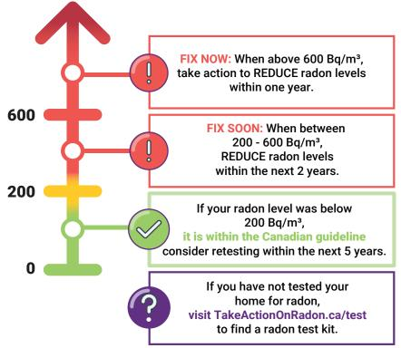
Radon gas levels are reduced the most by installing a radon mitigation system. Research shows that certified radon professionals can reduce levels by over 90%. Other steps, such as increasing ventilation and sealing cracks, can help in the short-term but are less effective.
