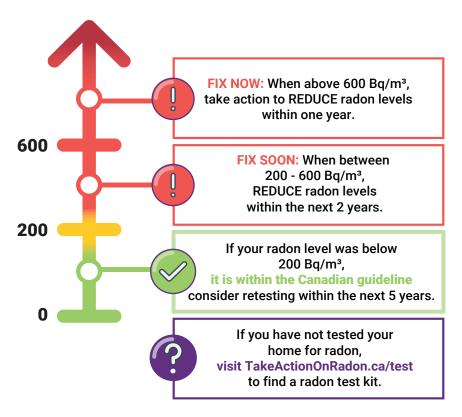
Radon gas levels are reduced the most by installing a **radon mitigation system**. Research shows that **certified radon professionals** can reduce levels by over 90%. Other steps, such as increasing ventilation and sealing cracks, can help in the short-term but are less effective.
