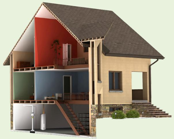
The BC Building Code requirements for radon vary by year and region. Some homes have a radon stub pipe or an extended pipe that runs through the house. These features are the beginning of a radon mitigation system and can make installation easier. Long-term (91 day) testing is still necessary.
